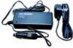
**Procat Fast Charger:** This fast charger is for the Procat boat batteries. It will fast charge the battery either from the mains at home or from a leisure/ car battery. The charger changes from bulk charge to trickle charge automatically and will charge a Procat boat battery in approximately 2 hours.
